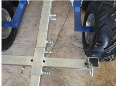
8.) Slide the cage over the inner frame rail. Installed right up against front frame portion. Install 2 large bolts and tighten.
