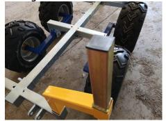
14.) The finished trailer should look like this. You can now adjust the inner frame and cage to extend or shorten the overall length of the trailer.
