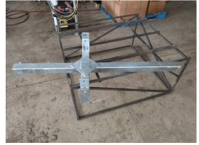
3.) Place the walking beams between the tabs on either side. The holes drilled in the walking beams are offset, therefore one end is slightly longer than the other. The short end of the walking beam will be facing the rear of the trailer. The front of the trailer has the bolt holes drilled on the side- as seen in the photo below. Install the large swivel pins, install the small bolts into the plate on the large swivel pins and install cotter pins on the backside. Grease both swivel pins
