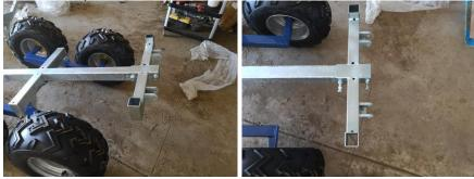
7.) Slide the front frame portion over the main frame. Slide it right up to the main frame. Install 2 bolts and tighten.
